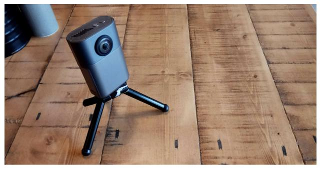
The camera is based on a Rockchip 1108 System on Chip (SoC) running Linux. Within its operating system, it raises three services to serve images and video, control the camera and stream video over a WiFi interface. In addition to these services, the camera presents itself as a standard webcam if connected via USB.
